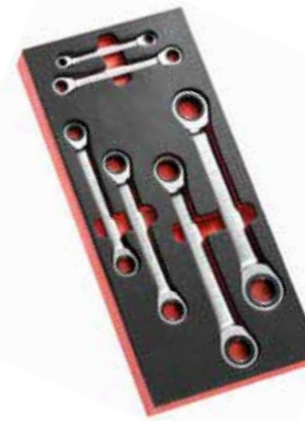
MODULE 6 STRAIGHT RATCHET RING WRENCHES - 12 POINT IMPERIAL MODM.64JU6 - 64.: 1/4 x 5/16 - 3/8 x 7/16 - 1/2 x 9/16 - 5/8 x 11/16 - 3/4 x 13/16 - 7/8 x 15/16" - Increment 5° - Foam tray : PM.MOD64JU6
