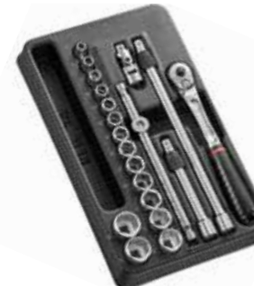
M MODULE 6-POINT SOCKET 3/8" - RATCHET MOD.JL171-36 - Sockets : JH. : 7 - 8 - 9 - 10 - 11 - 12 - 13 - 14 15 - 16 - 17 - 18 - 19 - 21 - 22 mm - JL.171 : ratchet 3/8" - J.210 - 215 : 2 extensions 125 and 250 mm - J.240A : cardan - J.120A : sliding tee - Thermoshaped inlay: PL.M15 Dimensions: 31 x 18,8 x 3,7 cm
