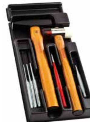
MODULE BLOW TOOL, HAMMER HICKORY 205H MOD.M13 - 205H.50: hammer DIN Hickory 500G - 208A.32CBA: plastic hammer (steel 32 mm) - 263.18: cold chisel - 256.6: center point - 248.: 4 - 5 - 6 mm: 3 long punches - Thermoshaped inlay: PL.333
