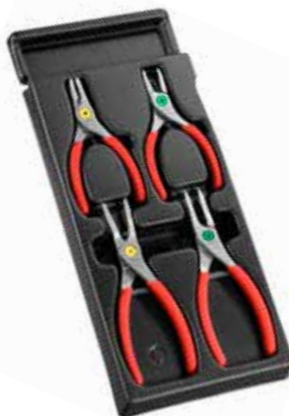
MODULE OF 4 CIRCLIPS® PLIERS MOD.PCSN - 177A.13 : Straight external pliers 10 - 25 mm - 177A.18 : Straight external pliers 19 - 60 mm - 179A.13 : Straight internal pliers 12 - 25 mm - 179A.18 : Straight internal pliers 19 - 60 mm - Thermoshaped inlay: PL.683
