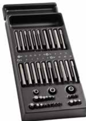
MODULE 41 LONG BITS AND SHORT 3 SOCKETS BIT HOLDERS MOD.E41 Hexagon: H.2L: 4 - 5 - 6 - 7 - 8 - 10 mm EH: 4 - 5 - 6 - 7 / EH.2: 8 - 10 mm XZN: EV.2L: 5 - 6 - 8 - 10 mm / EV.: 6 - 8 - 10 mm Torx®: EX.2L: 30 - 40 - 45 - 50 / EX.2: 45 - 50 - 55 Resistorx®: EXR.1L: 10 - 15 - 20 - 25 - 30 - 40 EXR.1: 10 - 15 - 20 - 25 - 30 - 40 Pozidriv bits: 1-2-3 - S.J.236: socket bit holder 5/16" - R.235: socket 1/4" bit holder - S.236: socket 1/2" bit holder 5/16" - Thermoshaped inlay: PL.621 Weight: 0,895 kg
