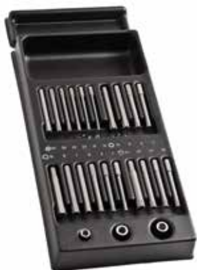
MODULE WITH 20 SCREW BITS MOD.E20L Hexagon: EH.2L: 4 - 5 - 6 - 7 - 10 mm XZN: EV.2L: 5 - 6 - 10 mm Torx: EX.2L: 30 - 40 - 45 - 50 Resistorx: EXR.1L: 10 - 15 - 20 - 25 - 30 - 40 S.J.236: cap CDX bit holder 5/16 R.235: socket 1/4" bit holder S.236: socket 1/2" bit holder 5/16 - Thermoshaped inlay: PL.624 Weight: 0,755 kg
